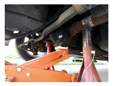
3. Removing the brake cable is pretty simple, just use the flat head screw driver as a lever to free the tension of the cable.
