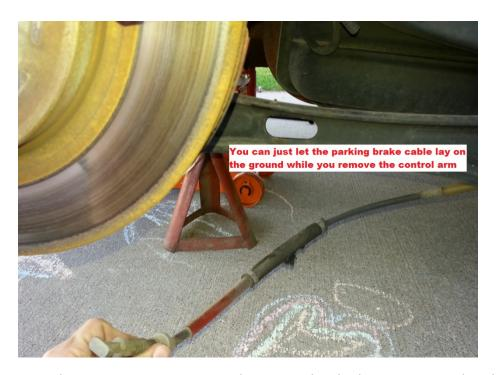
4. Remove the rear control arm using an 18mm wrench. Start with side that is connected to the car.
