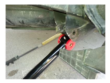
Getting the new control arm into place can be a little work; the red bushings are a pretty tight fit. I ended up using my jack with some padding on it to jack the control arm up into place. For small incremental adjustments I used a rubber mallet. Begin with the front bolt, once the front bolt is in, make sure you DO NOT tighten it all the way, that way you can more easily maneuver the control arm to get the rear bolt in.
