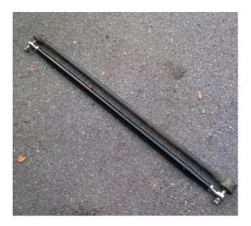
3. Now you are ready to install by placing the driver's side joint into place using the supplied washer (shown with arrow), if able to fit. Insert the bolt through the bushings and thread the nut on but do not tighten yet.
