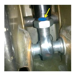
\*\*If you cannot get a wrench to fit inside of the bracket to tighten the passenger side nut, you will have to get it adjusted where you want it and remove both of the bolts and drop the panhard bar, tighten the nut on the ground with a wrench and then re-install.\*\*
