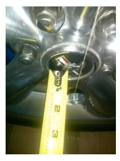
6. To adjust the length of the bar, you can spin any part of the black portion one way or the other. Both nuts on each side need to be loose to do this. Counter-clockwise from this view shown (driver's side) will lengthen the bar, which will move the axle to the left. Moving the bar clockwise will move the axle to the right.
