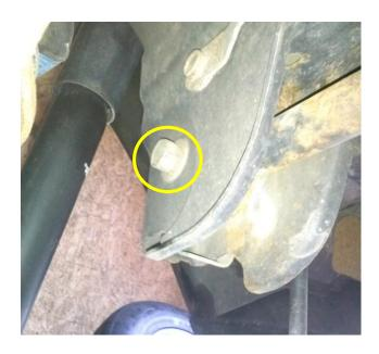
4. You will probably need a pry bar at this point to pry the old panhard bar out of the housings on either side and remove from the vehicle.
