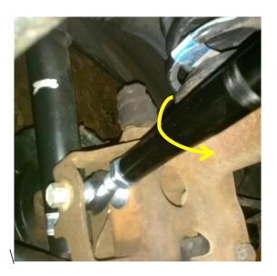
7. After you are satisfied with the adjustment, you can tighten the nuts with a 24mm wrench. Before tightening apply a small dab of blue Loctite to the threads (shown in picture). The driver's side nut is easy to get to; the passenger's side is a tight fit because of the surrounding bracket that gets in the way
