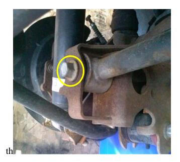
3. Then remove the passenger side bolt using the 18mm socket and ratchet
