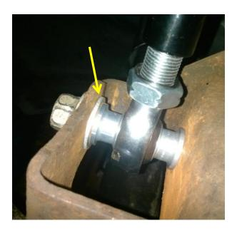
4. You can now swing the passenger side of the bar into place. Pass the bolt through and hand tighten with a ratchet using the 18mm, as well as the bolt on the driver's side. Final torque should be done once the vehicle is on the ground.
