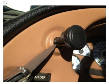
**STEP 3:** Remove the (2) 8mm nuts that retain the headlight switch in the car. Press down on the silver button and pull out on the shaft to release it from the headlight knob.
