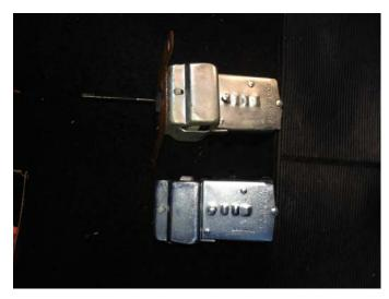
**STEP 6:** Unscrew the plastic nut retaining the mounting bracket and move both to the new headlight switch. Reinstall everything and reconnect the battery cable.
