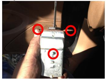
**STEP 4:** Unplug the headlight switch by pulling out on the two clips.
