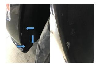
Once you have the screws removed grab the inner splash shield and pull out from behind the bumper cover to access the bolts holding the bumper cover to the fender.
