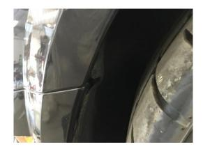
Remove the two 10mm headed nuts holding the cover to the fender. One can be seen in the picture, the second is just ahead of the one seen. Repeat for the other side.
