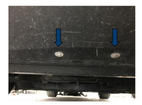
On each side in the fender well, toward the bottom of the bumper cover, there are three Philips screw head screws. These require removal. I used a Philips socket bit and ratchet to remove them. If you only have a screw driver, and cannot get it between the cover and tire, you will have to remove the front tires to remove them. These three screws are on each side.
