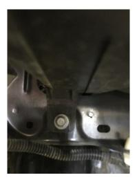
After the bolts and clip are removed, unhook the electrical connector, by pushing inward pressing the release tab, and pulling apart.
