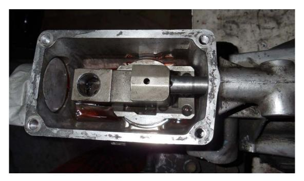
5. Remove the (8) 15mm bolts that hold the tail shaft to the Transmission Case (4 each side).
