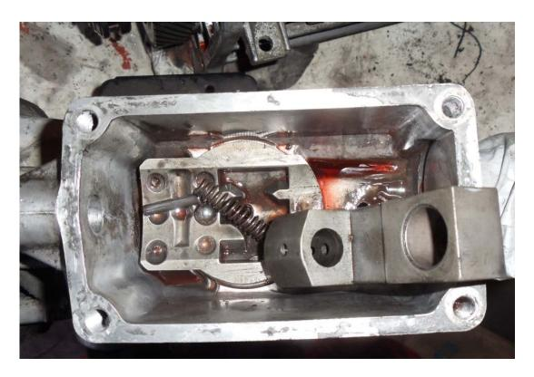
7. To remove the old Speedometer Drive Gear, pull the black bushing out. Then, you will have to push the retaining clip down while you pull the drive gear out. Be careful not to break the retaining pin.
