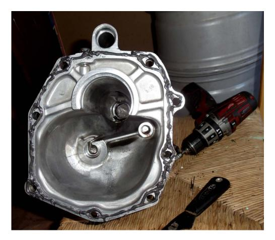
11. When reinstalling the tail shaft, **BE CAREFUL NOT TO BREAK THE SYNCHRONIZER CONE and REVERSE BRAKE**. You will have to put the tab at the 1 o'clock mark by turning the output shaft.
