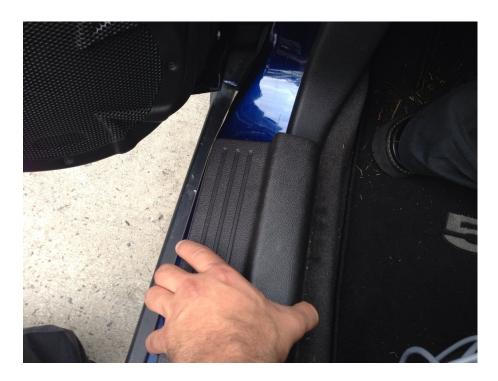
4. Remove the panel cover that goes up the trim of the door and covers the engine latch handle and also remove the panel that has the hole for the window vents. They can be easily removed by pulling on them gently.
