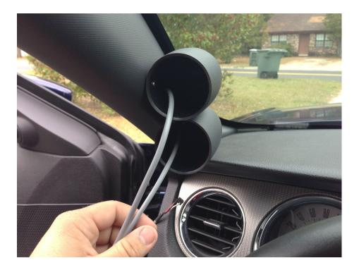
7. Plug in each gauge and the feed the cord back down towards the ODB2 port. Do it for both gauges. Push in the Aeroforce Gauges into the pod or gauge mount. If it's not secure, you can use soft Velcro, some tape, a piece of zip strip, etc... in order to make the fitment tight.
