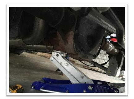
10. Jack up rear end until the control arm mounting holes line up to the axle mount and reinsert bolt.11. Double check to ensure all bolts has been re-tightened and lower vehicle.
