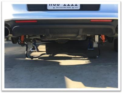
1. Lift the vehicle and place jack stands under the chassis (not rear axle).
