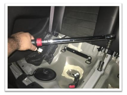
9. Insert the supplied M16 bolt and washer into the upper front hole located inside the car and tighten to 129 ft lbs, then reinstall the rear seat.
