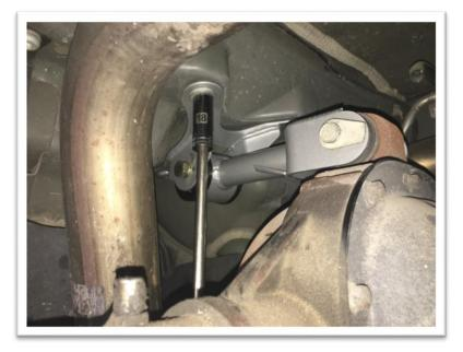
8. Bolt the mount to the car using the lower factory bolts and tighten to 110 ft lbs.
