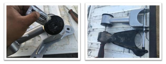
7. Prepare Whiteline Arm and Mount for installation by adjusting pinion angle of eccentric crush tube to desired position. Then tightening the lock nut up against the mount.
