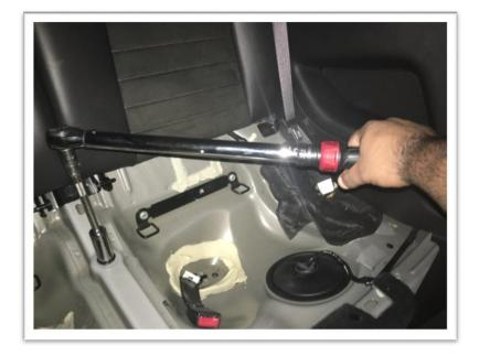
3. Remove the mount retaining bolt with a 18mm socket. (This is very tight so a breaker bar is useful)
