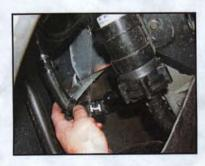
Disconnect the heat exchanger outlet hose from the engine. It is connected to a steel line just below the A/C compressor. You will disconnect the lower of the two hoses.
