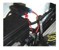
36) Run the wiring harness along the engine side of the fuse box up to the passenger side of the radiator. The harness will then go through the radiator support by the horns.
