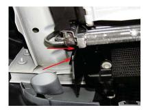
17) Using a 13mm deep well socket, remove the two bolts closest to center on each side that attach the front bumper to the frame.
