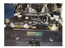
Remove the coolant tank cap from the heat exchanger coolant tank.
