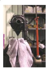
24) Connect the supplied 90° rubber hose between the pump outlet (facing down) and the heat exchanger inlet (30° tube). Trimming of the hose may be required. Clamp both ends with the supplied hose clamps.
