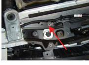
38) Remove the plastic loom on the coolant pump harness and locate the white wire. This wire will have battery voltage when the pump is activated. Cut this wire approximately 2" from the pump connector.
