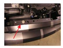
10) Lift the top of the bumper up and over the tabs. Then, slide the whole bumper cover forward and off of the vehicle.
