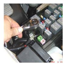
34) Place the red wire from the fan harness on top of the power lead previously removed and bolt back into place. Remove the bolt next to the fuse box and mount the relay as shown.
