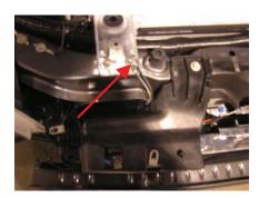
37) Remove the plastic loom on the coolant pump harness and locate the white wire. This wire will have battery voltage when the pump is activated. Cut this wire approximately 2" from the pump connector.
