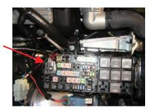
33) Place the red wire from the fan harness on top of the power lead previously removed and bolt back into place. Remove the bolt next to the fuse box and mount the relay as shown below.
