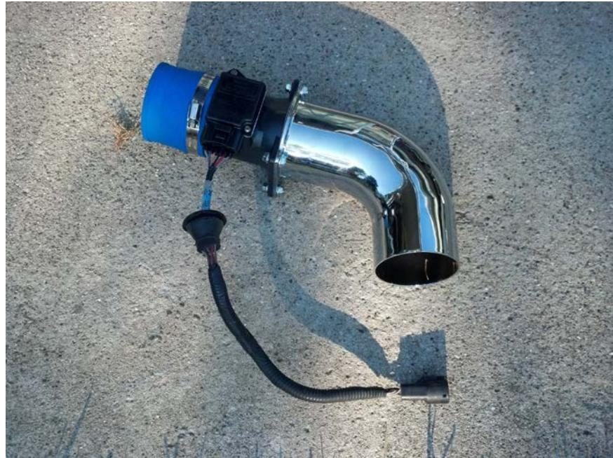
9. Before you install the filter, attach the heat shield to the lower intake pipe. The filter that is supplied with this kit must be installed from under the car because it is too big to be put through the pre-existing snorkel hole. Once the filter is in place and the pipe is attached to it, be sure the hose clamp is tightened down securely as you will not have access to it after the install is complete.
