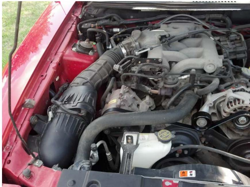
2. Next, unhook the connection to the Mass Airflow Sensor. This can be made easier by using a Flat Head Screwdriver to hold down the clip while you pull the connection out.
