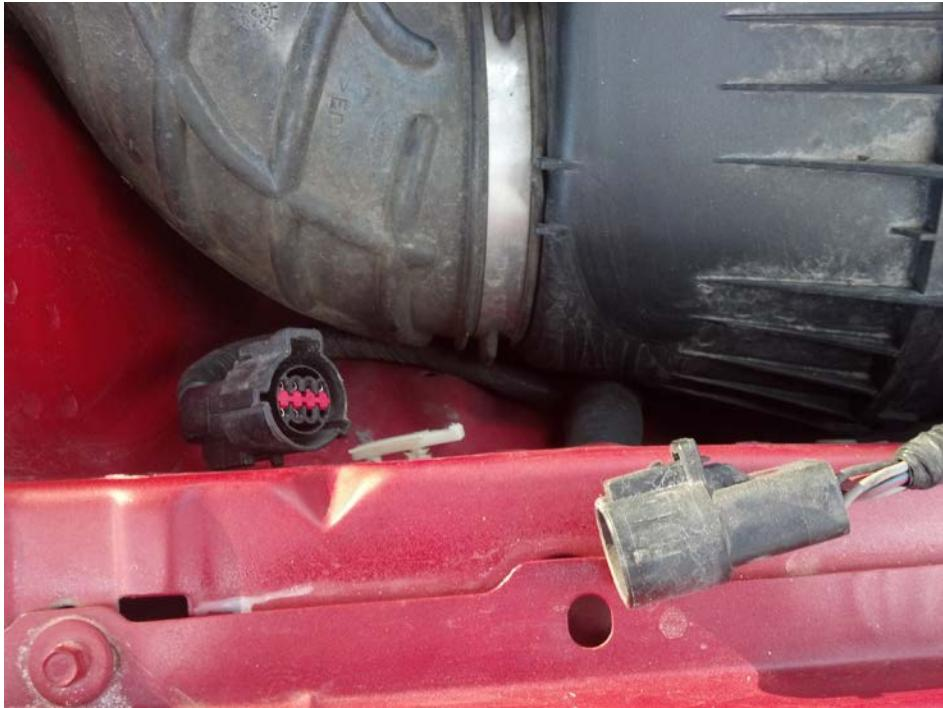
3. After you have the connection unhooked, you can now start to remove the stock intake by using an 8mm Wrench or Socket Wrench to loosen the bolt that's securing the intake to the fender. Also, unlatch the two clips holding the Mass Airflow Sensor housing to the stock snorkel.
