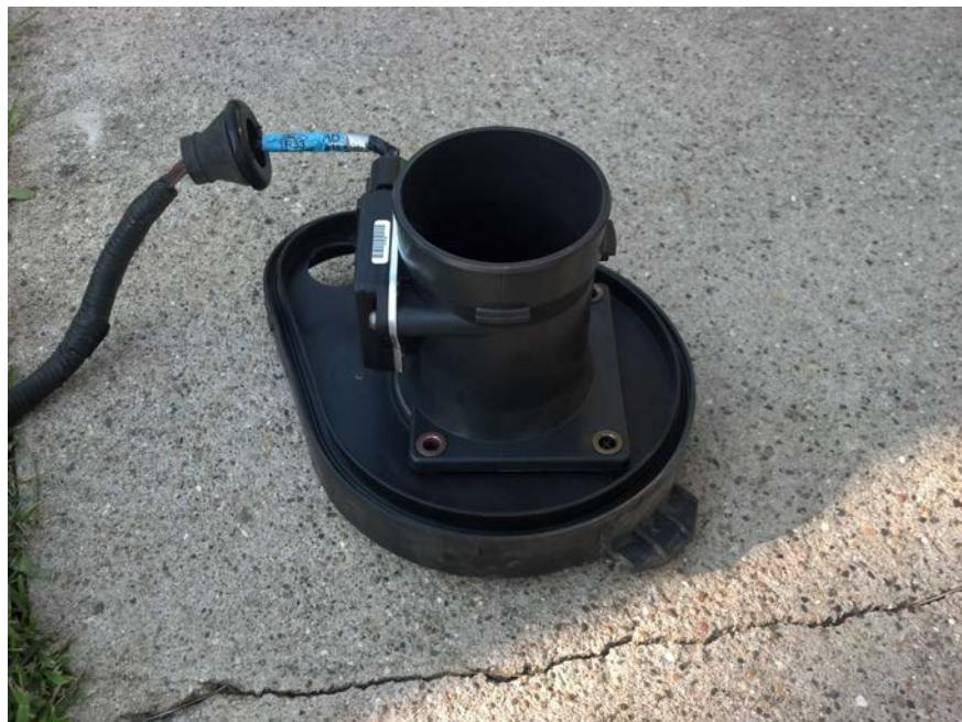
8. Next, attach the Mass Airflow Sensor to the lower intake pipe with a gasket separating the two pieces (this kit does not include the gasket so I made one with gasket material). Tighten the Sensor to the Pipe with the supplied bolts and lock nuts. Attach the remaining silicon coupler to the Sensor and tighten the hose clamp down. The assembly will now look something like this:
