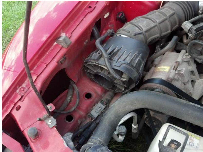
You may have noticed that one or both rubber grommets came out of the holes under the snorkel, just take them off of the stock intake and put them back in. At this time, install the aluminum mounting hardware for the new intake.
