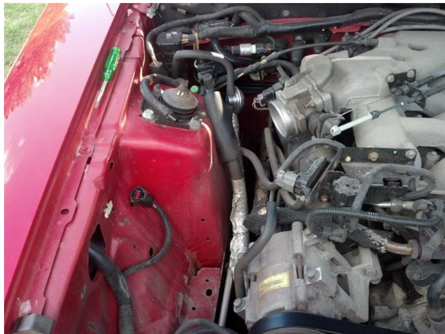
6. After the stock intake is completely off, installation of the new Cold Air intake can begin. Begin by taking the upper intake pipe of the new kit and fitting the smaller of the two silicon couplers to the Throttle Body and upper intake pipe. Tighten the hose clamps down just enough to hold things in place, as adjustments may be needed.
