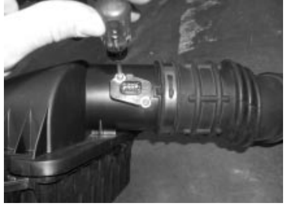
Remove mass air meter.
