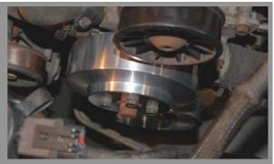
Install the BBK underdrive pulleys to the water pump and vibration dampener using the stock bolts.
