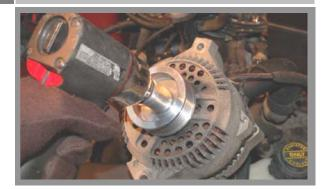
Remove the alternator mounting bolts, lift the alternator out of its cradle to access the pulley.
