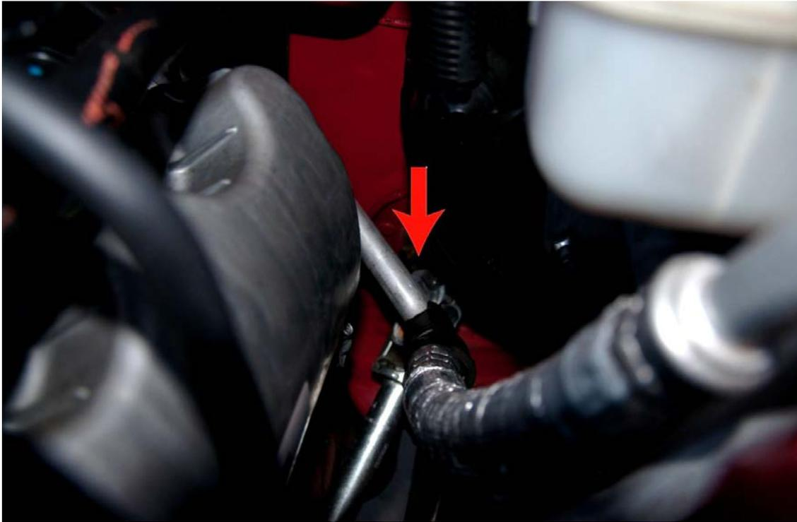
**Step 7** – Now that you have removed the H-pipe and steering shaft, it is now time to lift your engine to gain better access to the bolts on the starter and stock headers. Lifting the engine also makes the long tube header install easier as space is limited. Unbolt the (2) motor mounts (shown below) and use your jack to SLOWLY raise the engine. If you have a strut tower brace, remove it. Also, you may want to separate your intake from the throttle body as a precaution.
