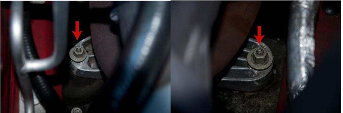
**Step 8** – Raising the engine. I found that the ideal location to lift the engine is by placing a block of wood towards the front of the engine block near the flywheel and slowly lifting the engine to the point at which the mount just clears the bolt it was bolted to.
