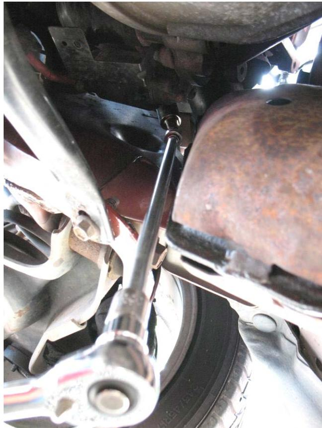
**Step 4.** Locate the 2 muffler clamps at the rear of the H-Pipe where it meets the muffler. Remove the bolts from each clamp using your Ratchet and Socket. There are (2) nuts and bolts on each muffler clamp. Once removed, set them aside in a safe location.
