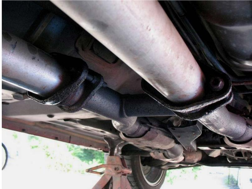
**Step 5.** Slide the hangers attached to the stock H-Pipe off of the rubber mounts and completely remove the H-pipe from under the car. Set aside the stock pipe where it will be out of your way.
