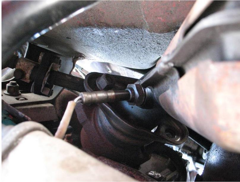
**Step 3.** Locate where the stock H-Pipe bolts into the Manifold at the front of the car. Use your ratchet and 18mm socket along with any extensions necessary to remove the nuts from the studs in the manifold. There are 2 nuts on each pipe. Once removed, set them aside in a safe location.
