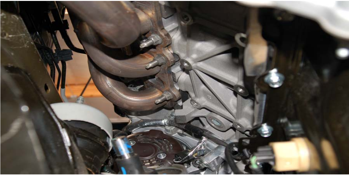
Fig 1. Motor Mount removed. Shows nut access.
