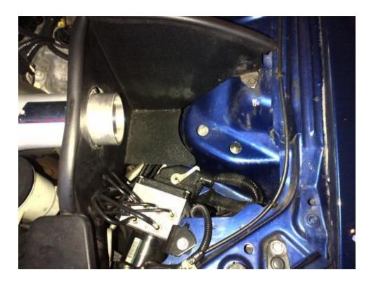
4. Also, take this opportunity to check inside the air intake. Check for dirt, debris, etc... If there is anything, clean out the air intake thoroughly. You may wish to remove your entire cold air intake (if its dirty) and clean it as this is the air that is going into your engine.
