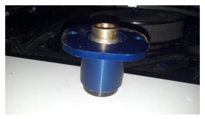
8. Use a rubber mallet to drive the bushing sleeve all the way in so it is even with the bottom of the strut mount and the top of the bushing sleeve is touching the bottom of the upper bushing.
