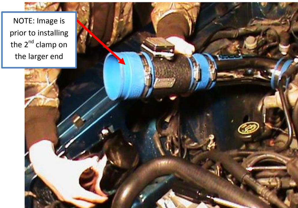
6. Bring the lower filter pipe together with the larger O-ring attached to your BBK Mass Air Meter and tighten the hose clamps into place. **NOTE:** Image below does not show the final clamp in place yet.
