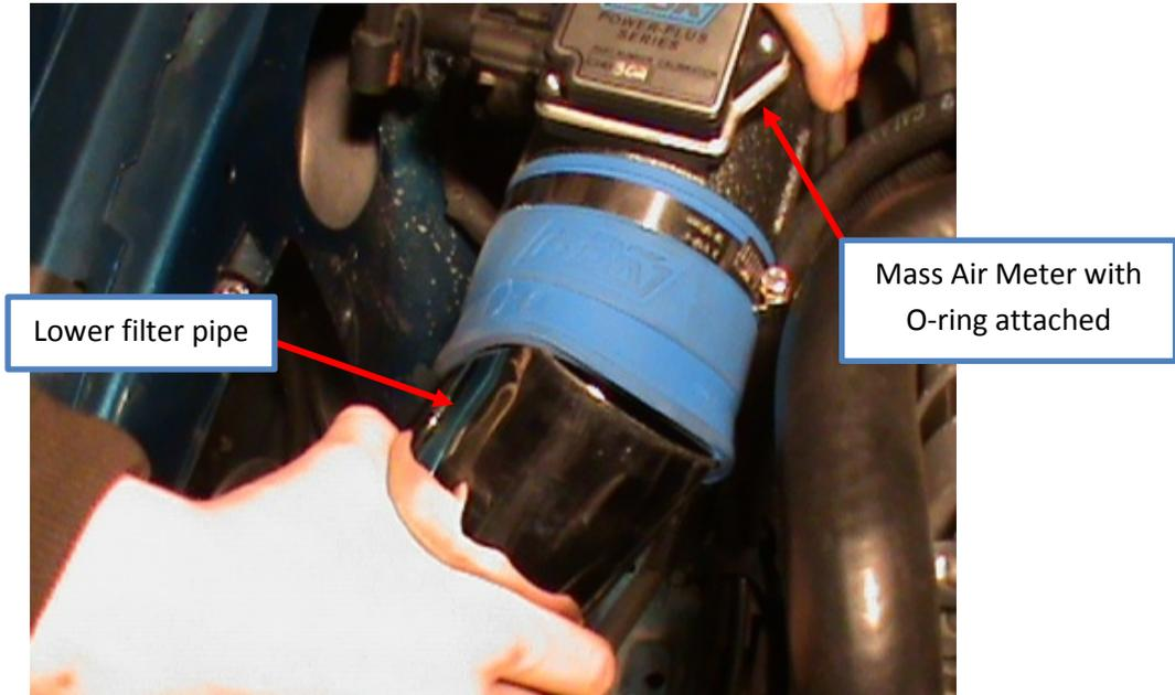
7. Tighten down all hose clamps completely at this time.
