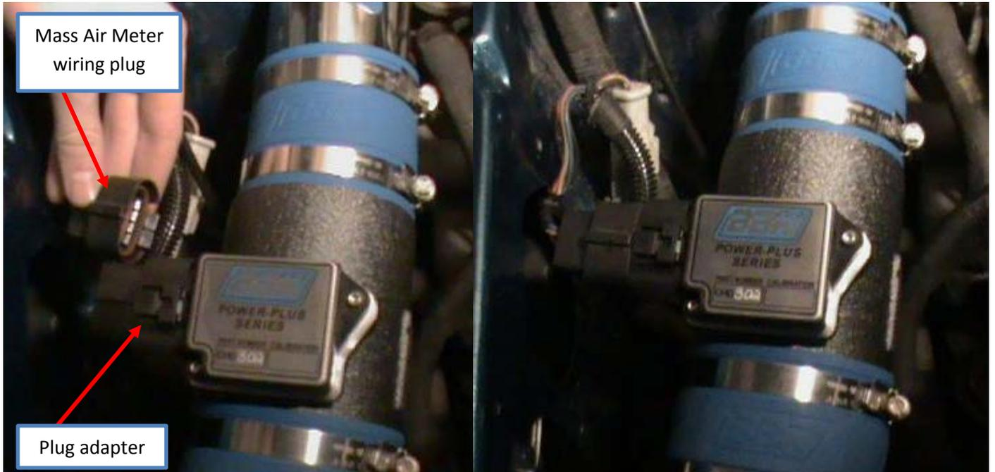
9. With the engine running, check for any leaks in the O-rings around your Throttle Body and Mass Air Meter.
