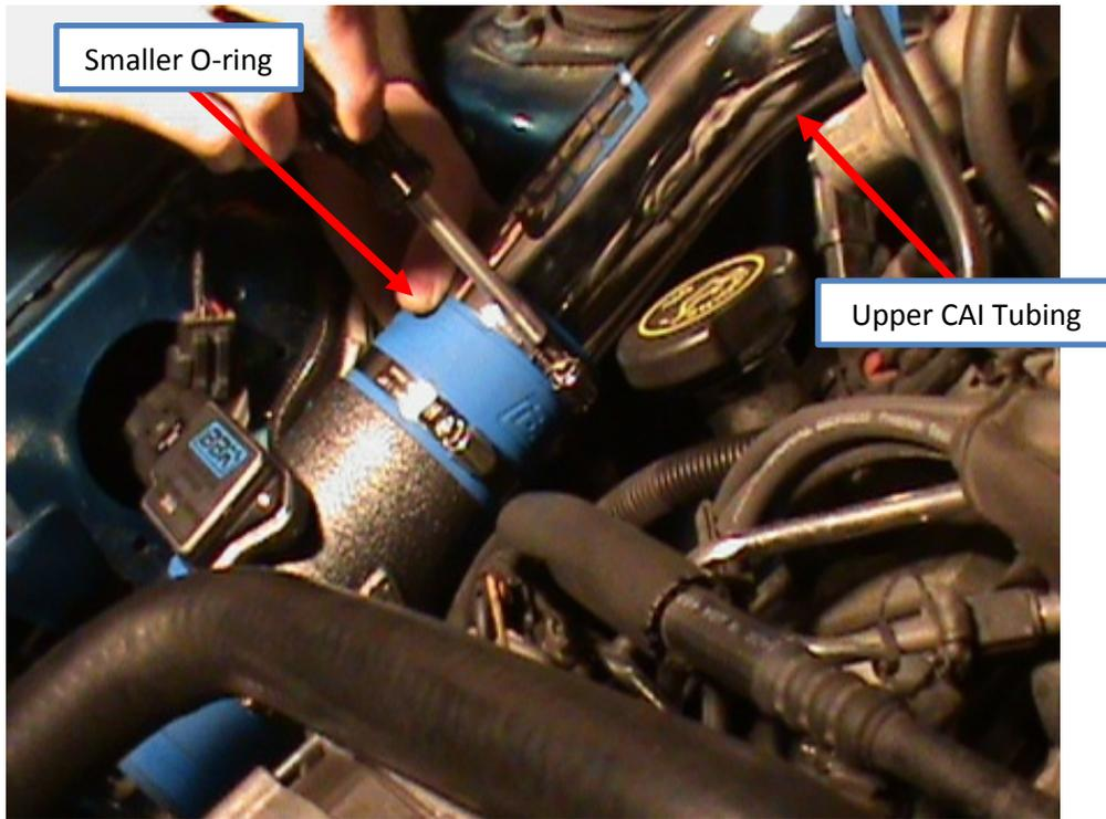
5. Move your upper intake pipe with Mass Air Meter attached to a slightly up-angled position. Do the same with your lower filter pipe.
