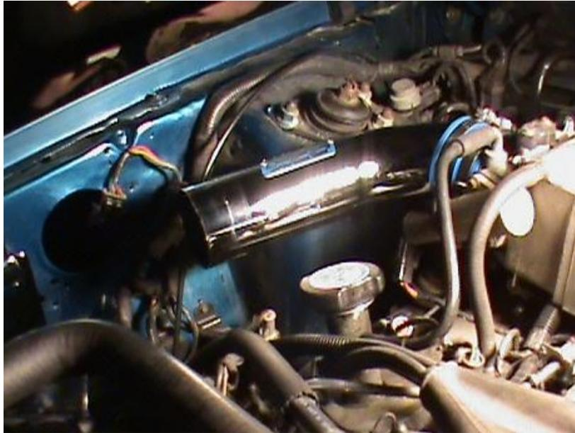
2. Using the image below for reference, slide the O-rings onto either side of your BBK Mass Air Meter; smaller on TB side and larger on air filter side. Slide on your (4) hose clamps and tighten down snugly so they don't fall off, but not completely using your flathead screwdriver.
