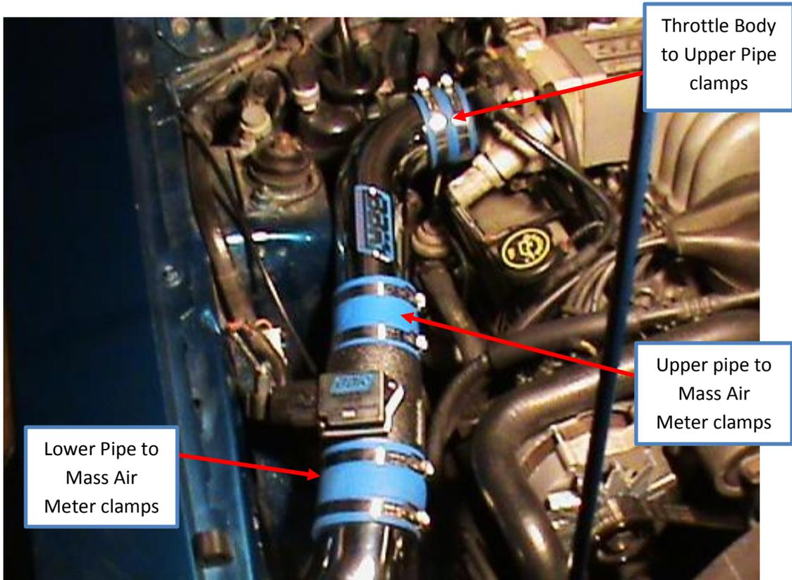
8. Plug the wiring harness back into your BBK Mass Air Meter using the adapter that came with the Mass Air Meter and be sure it clicks into place.
