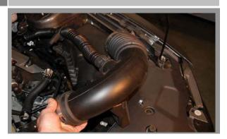
Loosen the clamps on the air inlet tube at the air box and the throttle body. Remove the air inlet tube and set it aside.
