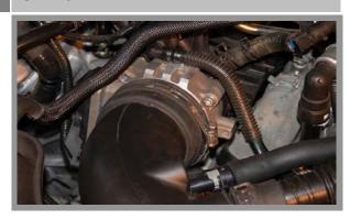
Re-install the air inlet tube and reconnect the breather tube. A little WD-40 or light grease on the inside of the tube may help in this process. Tighten Clamps.
