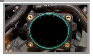
Wipe off the stock rubber throttle body gasket to remove any oil or debris. You will be re-using this gasket.
