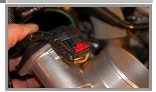
Remove the 4 mounting bolts from the stock throttle body, as you remove the stock throttle body; flip it to disconnect the motor plug on the bottom.
