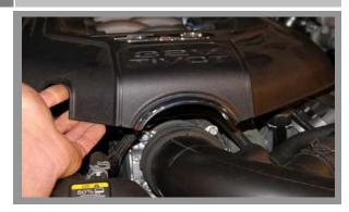
Remove the engine cover by pulling up on it to release its mounting pins from the grommets on the intake manifold.
