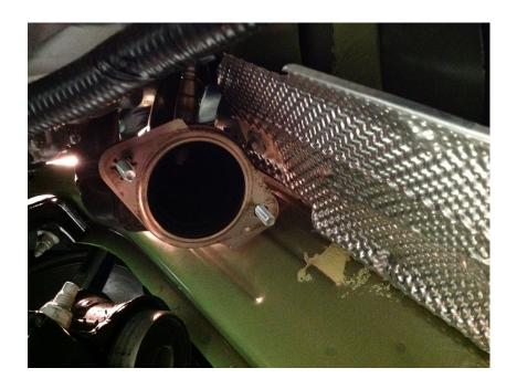
14. Install BBK pipe onto factory manifold. Do not tighten fully at this point:
