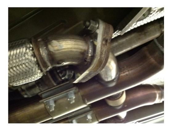
6. Loosen bolt holding exhaust exit to body
