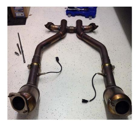
10. Loosen clamps securing catalytic converters to the mid pipe and remove cats using a 13mm wrench. This may be easier to prop up the pipe and tap catalytic converter with rubber mallet:
