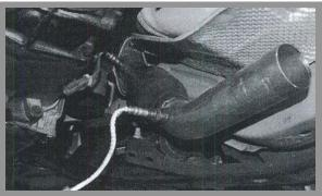
Carefully remove the complete mid pipe section.
