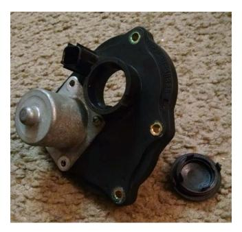
9. Place the capped spring that popped out earlier over the throttle body shaft and twist it until the pigtail at the end of the spring is inside the slot of the gear.
