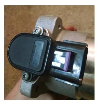
14. Install the throttle body back onto the engine and tighten the 4 bolts evenly to a torque of 89 **INCH/LBS**. (Or 8 ft/lbs) The SR kit comes with two new 5mm Allen bolts to replace the two upper studs, however the factory engine cover would not be able to be secured with these.
