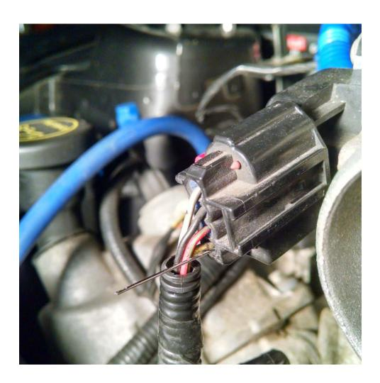
4. Attach the black ground lead to a suitable ground (I used the negative battery terminal) and record the voltage with the **KEY ON, ENGINE OFF.**
