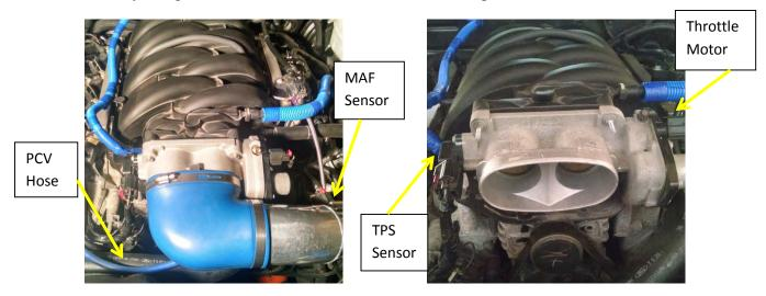
2. It is then recommended to get a voltage reading from the signal wire (yellow color) on the Throttle Position Sensor (TPS), located on the passenger side of the throttle body. If this isn't done now, the Check Engine light may come on after the install and the stock throttle body will need to be re-installed and this reading taken.
