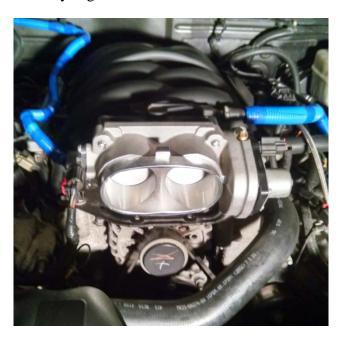
15. Install the TPS connector, the electric motor connector, and the intake tube and tighten all clamps.
