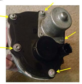
7. Next remove the two T20 screws holding the TPS sensor in place and carefully remove the sensor being careful not to let it rotate.
