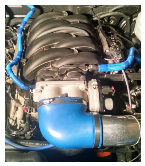
16. Connect the MAF connector and PCV hose. Enjoy the extra new horsepower and throttle response!
