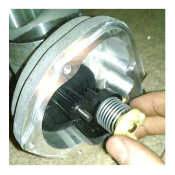
10. Install the motor housing, without the black circular cap, onto the throttle body over the plastic capped spring and tighten the 5 screws.
