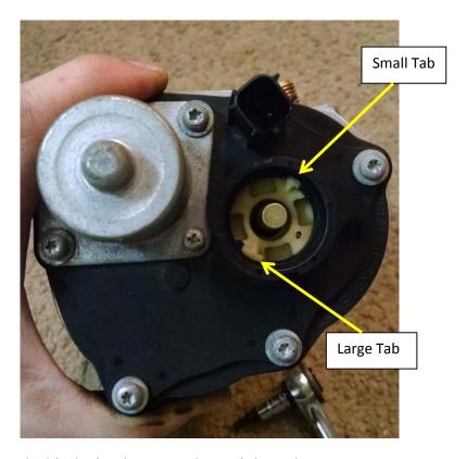
12. Align the tabs on the black circular cap and snap it into place.
