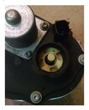
11. Use needle nose pliers to push down slightly and rotate the plastic spring cap **COUNTER-CLOCKWISE** around half a turn until the small tab and big tab line up and it is able to slide up and lock into place.
