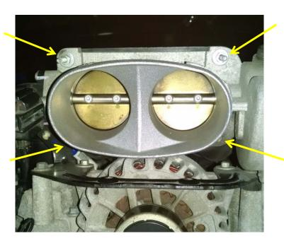
8. Use a T20 Torx bit to remove the 5 screws holding the housing in place, the 2 Phillips screws don't have to be removed. There is a capped spring inside the housing that will pop out and needs to be re-installed.
