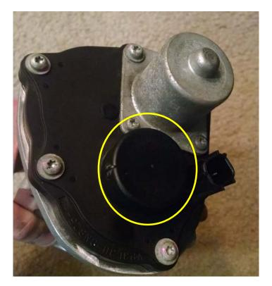
13. Push the TPS back into place being careful not to let the sensor rotate on the shaft and tighten the screws.
