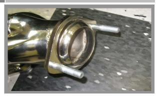
Install the supplied studs onto the BBK Header Collectors.
