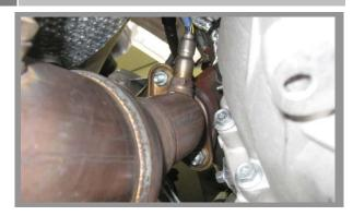
Unbolt the factory x-pipe from the exhaust manifolds and let it hang down. This will aid in tightening the passenger side BBK Header.
