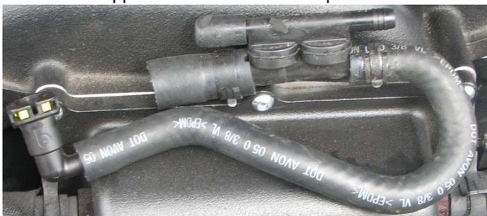
78. Route the rest of the supplied 3/8" brake hose along the driver side cylinder head and attach it to the fitting on the brake booster and secure it with a clamp.
