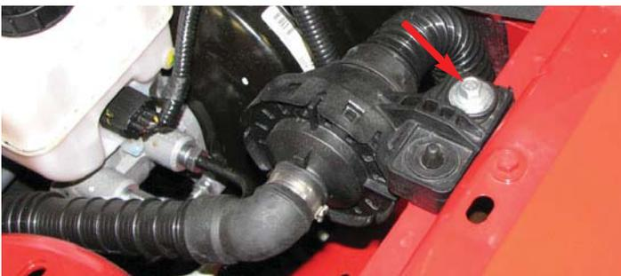
14. Loosen the throttle body and air box cover worm clamps then remove and discard the inlet tube assembly. Vehicles equipped with an automatic transmission will also need to detach the brake booster hose from the tube.
