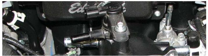
81. Install the stock throttle body on the nose inlet using the stock o-ring seal and bolts.
