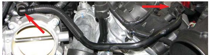
18. Remove the EVAP tube by detaching it from its retaining clips and hard line then set it aside for reuse.
