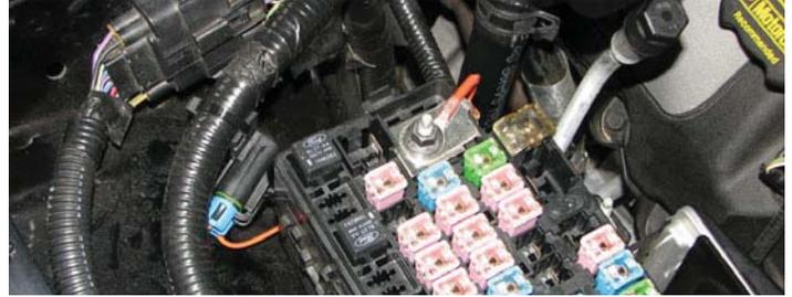
89. Route the water pump electrical connector below the fuse box and around the washer fluid reservoir and plug it into the intercooler water pump.
