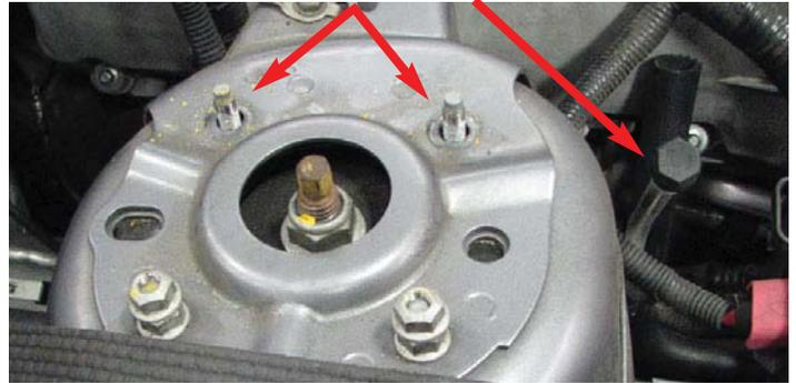
92. Remove the 10mm ground strap from the passenger side strut tower bracket and pull out the harness body pin. Route the strap to the ground stud on the outboard side of the fuse box and secure it with the nut supplied in Bag #7.
