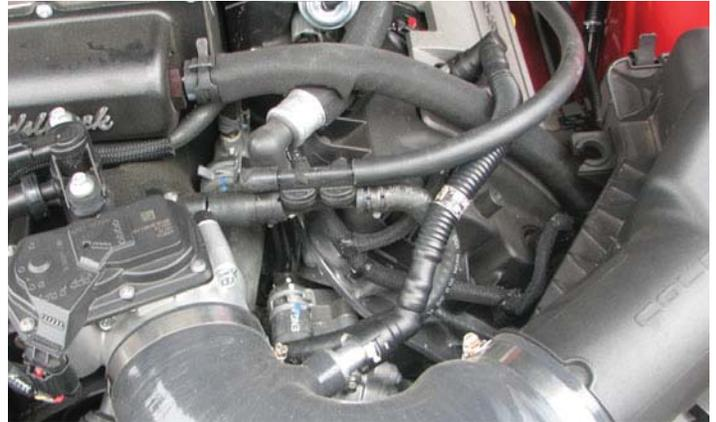
100. Plug the MAF/Temp wiring harness into the Temp sensor then route the rest of the harness along the inside of the driver side fender to the front of the air box.
