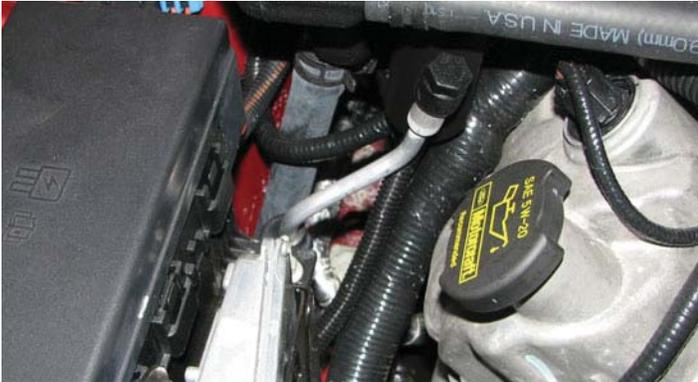
95. Install the short straight hose from the recovery tank to the passenger side intercooler fitting and secure both ends with the supplied hose clamps.
