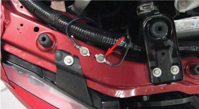
87. Route the longer wire harness segment under the fuse box and attach the fuse holder to the passenger side strut tower with a 10mm socket and the M6 bolt supplied in hardware bag #7. The large white electrical connector can be removed by sliding it to the right for easier access to the bolt. Replace the connector once the fuse holder is mounted.
