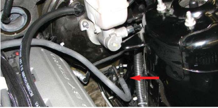
84. Install the stock driver side PCV hose onto the passenger side PCV fitting and attach it to the passenger side of the supercharger manifold.
