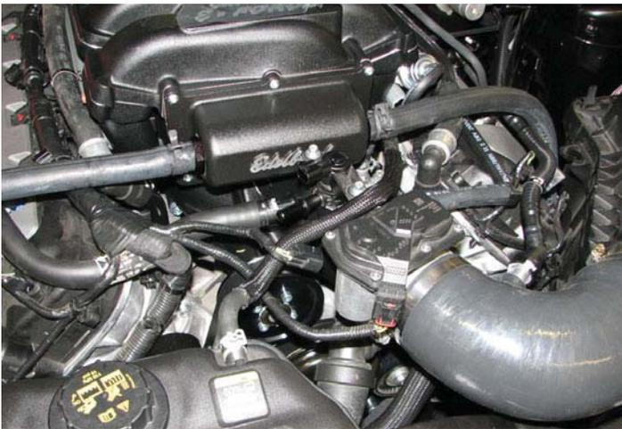
98. Owners of an automatic transmission vehicle will need to remove the cap from the fitting at the bottom of the throttle body elbow and attach the molded hose connected to the brake aspirator. Owners of a manual transmission vehicle *must leave the cap in place*.
