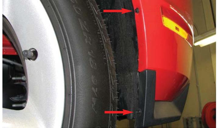
8. Remove the five push pins retaining the front half of both front wheel well liners. Note that the two top pins pass through both the front and rear liners. Remove the front half of the liner on both sides of the car.
