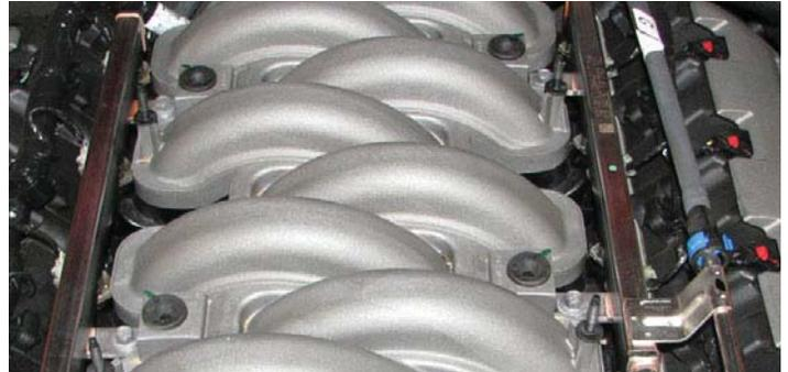
28. Use a 10mm socket to remove the four fuel rail bolts, then lift the injectors out of their provisions. The rails and injectors can be removed together and discarded.
