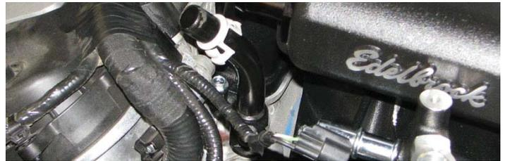
80. Install the stock EVAP solenoid on the provision at the top of the nose inlet using the stock bolts and o-ring.
