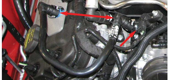
16. Disconnect the EVAP solenoid connector at the top of the throttle body flange on the manifold.
