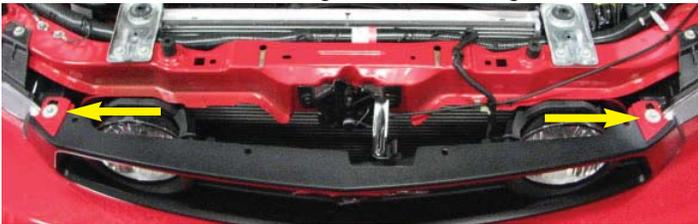
6. Raise the front of the vehicle using a jack and jack stands or a service lift. Remove the nine 7mm bolts retaining the lower splash shield. Pull down slightly on the shield to disengage the clips and remove it.
