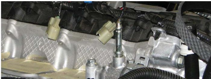
57. Remove the coil covers from the cylinder heads, then remove the ignition coils to access the spark plugs. Remove the plugs with a 5/8" spark plug socket and gap them to .034". Reinstall the plugs and torque them to 9 ft-lbs., then reinstall the coils and coil covers. Be sure to install the plugs and coils in the same spot they came off.
