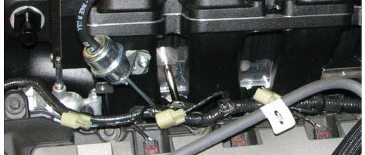
70. Lower the fuel rail assembly onto the supercharger and line up the fuel injectors with their provisions on the manifold. Push down on the rails gently until the fuel injectors are fully seated then install the four M6 x 30mm bolts supplied in Bag #1 to secure the rails.
