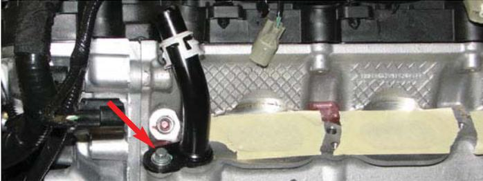
35. Use a soft cloth to remove any contaminants on the sealing surfaces of the cylinder heads. Use masking tape to prevent any debris from entering the exposed ports.
