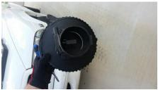
7. Now you will assemble the air filter to new 85mm MAF housing, then you will attach the new filter and housing to the intake tube.
