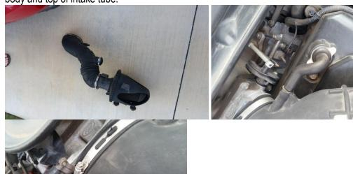
5. Take apart intake tube, MAF sensor and air box. You remove the air box from the intake tube then use Torx bit with screw driver to take out MAF sensor from old air box and old MAF housing.
