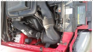
3. Remove bolt holding air box to inside of car with 5/16" wrench, remove shaker hose, and unplug MAF wire to MAF sensor.
