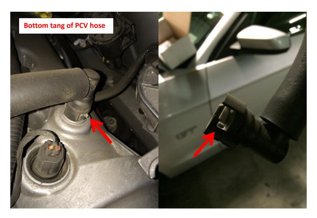
2. Install the JLT assembly connecting the straight end up top, and the angled end down on the bottom fitting over the valve cover. Assure both tangs are fastened securely in place
