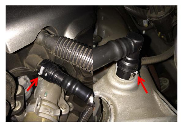
3. Start your Mustang and ensure the assembly is secured in place and there are no oil leaks through any of the connections
