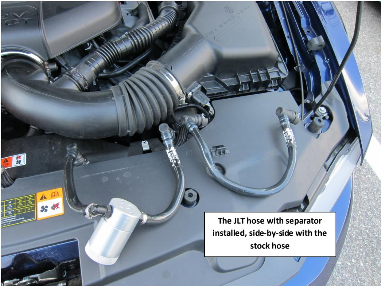
The JLT hose with separator installed, side-by-side with the stock hose
