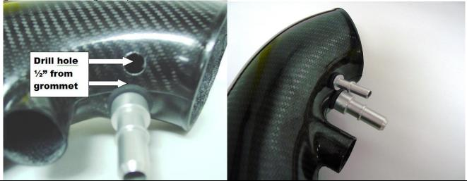
Attach coupler and clamps to the small end of the JLT tube and the air filter to the large end. Note; part#s
