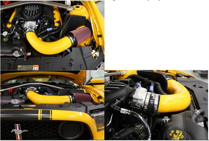
The sound tube brings engine noise into the cabin. Adding the intake will increase engine sounds and it may not be needed per your taste.
