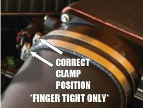
8 Squeeze the rubber air duct from the grille and insert fully into oval hole in heat shield.
