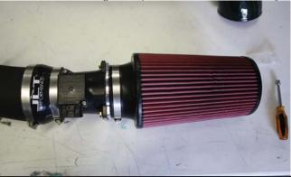
PULL the Inlet Air Temperature sensor from your stock inlet and install in the grommet on bottom side of JLT tube.
