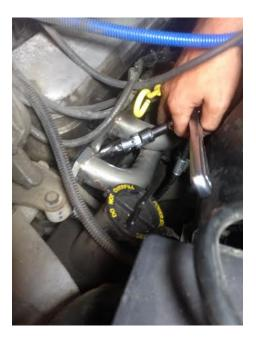
**Step 4:** Take the spark plug boot that was removed off the old plug and re install it on the new plug.
