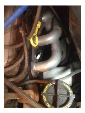
**Step 3:** With the 5/8 plug socket tighten the spark plug until its snug, give the plug another 1/16 to 1/8 of a turn. Do not over tighten
