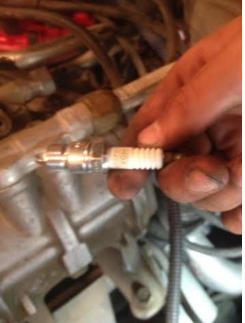
**Step 2:** Thread the new spark plug into the cylinder head.
