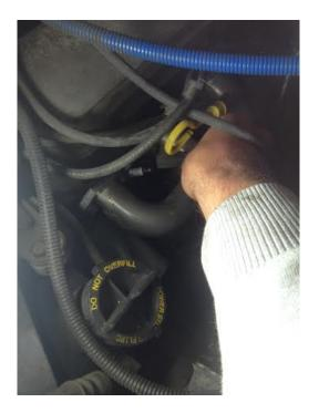
**Step 2:** Using the 5/8 spark plug socket remove the spark plug.
