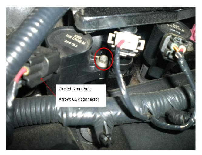
6. Remove the COP by giving it a wiggle and removing it from under the fuel rail.
