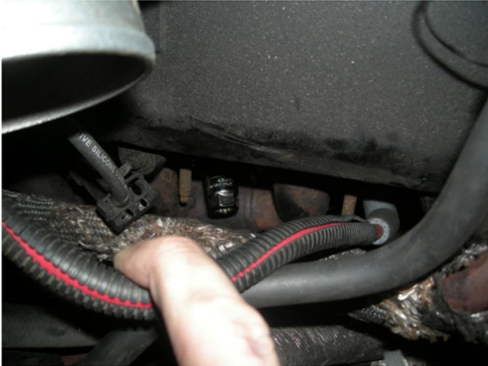
13. Once you have finished with the passenger side, I would recommend using some zip ties to hold the wires together so they are not all over the place. Then trim the extra off the zip tie.
