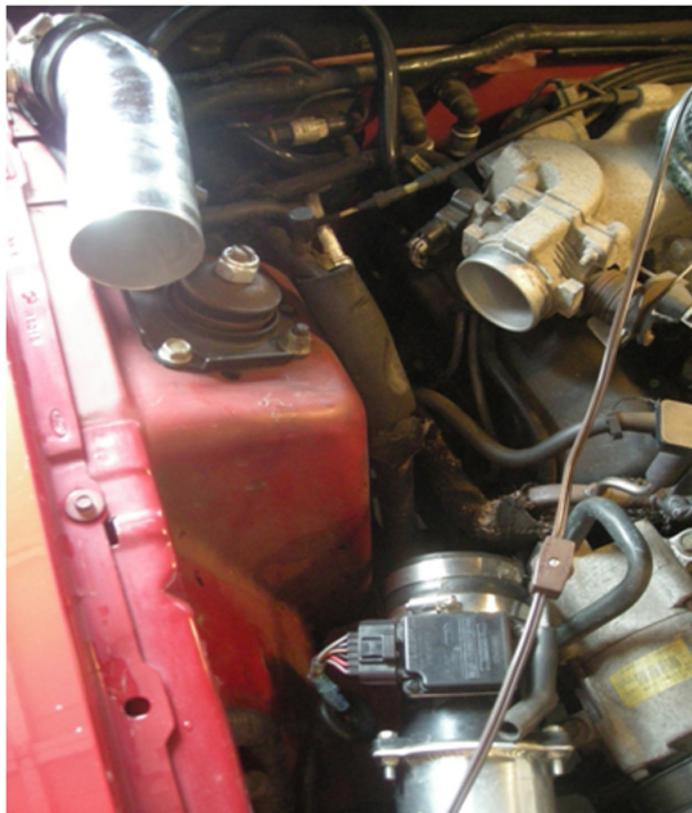
4. I started on the driver's side just because there is more space than the passenger side. Starting with the cylinder closest to the nose (front) of the car, locate and remove the spark plug boot from the spark plug. Follow it up to the coil pack and remove the wire completely.
