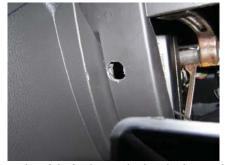
3. Unwrap the wiring attached to the switch and guide it through the hole, and push the switch into position. Sometimes it will need to be rotated slightly to sit flush on the dash.
