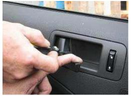
5. Remove the window switch plate assy. by prying up the top cover and gently pulling out the entire switch assy. almost horizontally. Remove the plugs from the switches and remove the assy.
