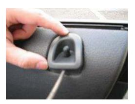
7. Using a 6mm socket, remove the (9) nine screws on the periphery of the door and the one hidden in the window switch area. See figure below for screw locations.
