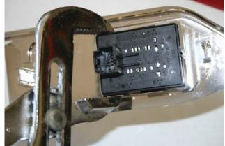
6. Using a small screwdriver or prying tool, remove the spring clips from the posts on the original door switch plate and transfer to the new switch plate. Install the new switch plate into the lower cover. Reconnect the wiring for the switches, temporarily turn the key to the on (but not start) position and test switches. If everything works well, reinstall on the door, using the alignment pins on the lower cover as a guide.
