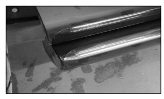
6.) Hold the rocker molding still and pull all 3 tabs beginning with the front of the vehicle as shown below. All tabs should pull in the same direction. Apply light pressure to the insert where the lining has been removed.
