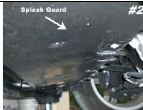
Black splash guard should be removed. It is held by 9 screws.
