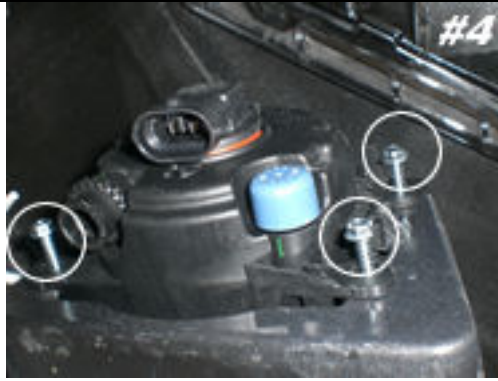
Drivers side fog light shown - looking upward from ground.
