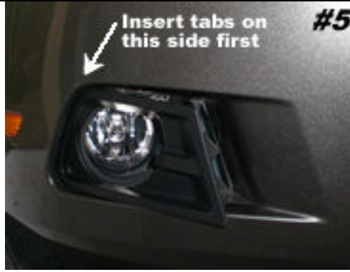
Passenger side fog light shown. Black bezel will snap into place.
