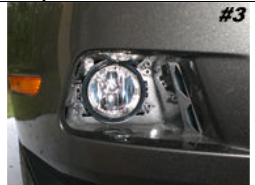
It is preferable to mount the lights with the bulb connector facing down.
