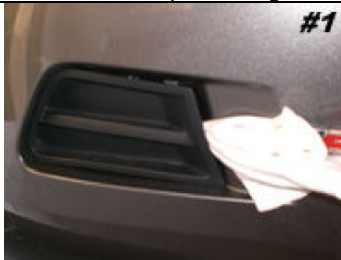
Gently pry the bezels out of bumper (passenger side shown).
