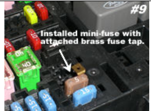
Make sure tan fuse is seated properly in fuse slot (position 39).
