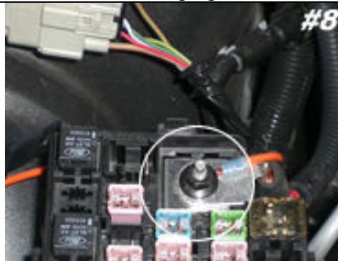
Be sure that the bolt is re-attached tightly enough that it will not loosen.
