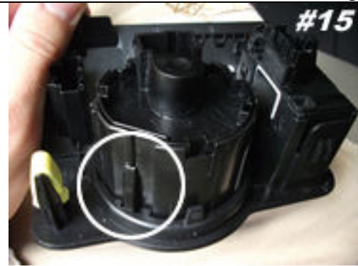
3 tabs hold switch in. One of the tabs is circled in the picture above.
