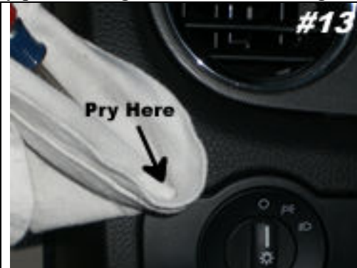
Pry up gently to loosen switch panel.
