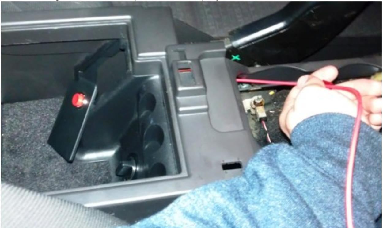
9. Locate the green and black wire running under the cup holder area towards the center console compartment. These wires plug into the 12-volt power supply located in your center console compartment. Place the supplied **Blue** wire tap onto the **Black** wire. The wire should sit in the middle of the two teeth. Squeeze down on the wire tap with a pair of pliers until it snaps closed. **DO NOT CUT WIRE!!!** Plug the **Black** wire from the button wiring into the back of the wire tap.
