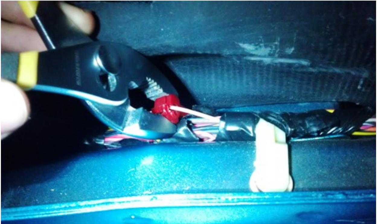
10. Finish routing the red wire down to the skid plate and plug it into the red wire tap. Tuck it in behind the kick panel so that it is out of view.
