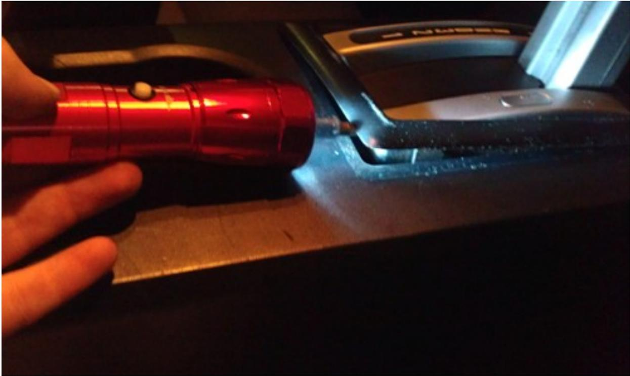
5. Begin to carefully lift the entire center console. Several clips hold the console into place and they will unsnap as you pull up on the panel.
