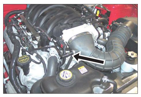
2. Loosen the clamps on both ends of the clean air tube and remove from the vehicle.
