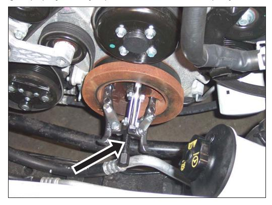
12. Remove the four water pump pulley bolts and pulley.
