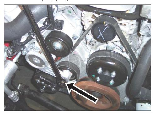
10. Remove the crankshaft pulley bolt and washer.
