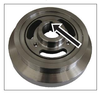
2. Using the special installation tool, install the new crankshaft damper pulley.
