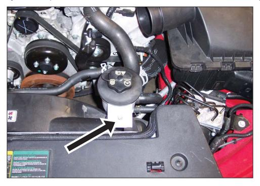
4. Remove the bolts holding the engine coolant reservoir to the fan shroud and fold out of the way.
