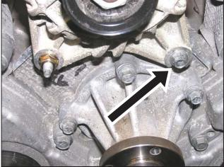
6. Install the new water pump pulley (R07020029) reusing the four factory bolts. Torque to 25 Nm (18.5 lb-ft).
