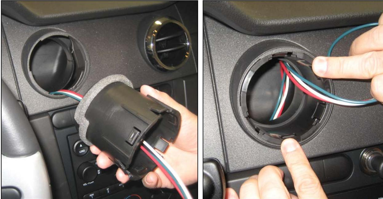
8. Feed the wiring through the VentPod and install the VentPod into the inner vent structure (see note below). Make all necessary wiring connections with the gauge as per the gauge manufacturer's recommendations. **NOTE:** Before installing the VentPod, orient the part such that any two of the support ribs align with the 12 and 6 o'clock positions (circled in RED) and press firmly in place.
