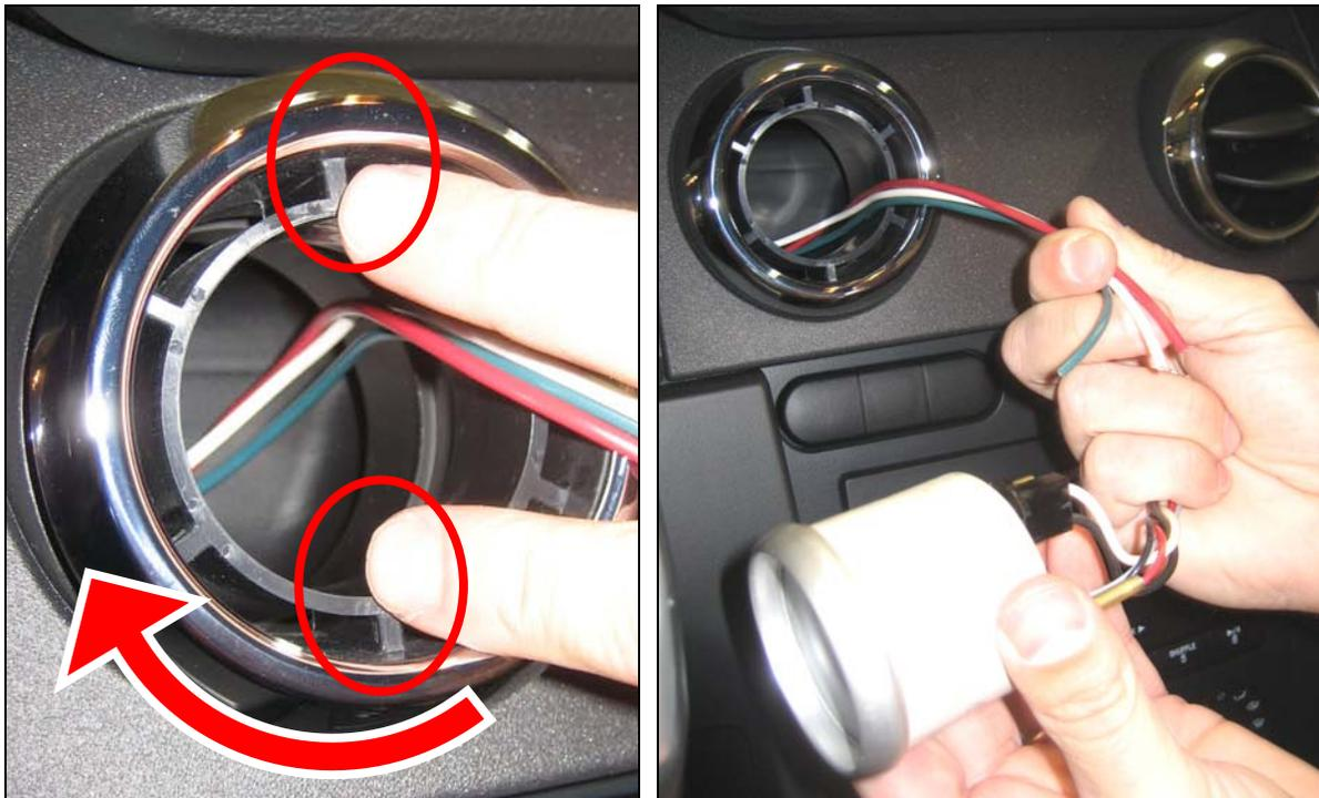
9. Insert the gauge into the VentPod and adjust the amount of “slack” wiring if necessary. Make all gauge hardware and vehicle connections as required as per the manufacturer’s recommendations.
