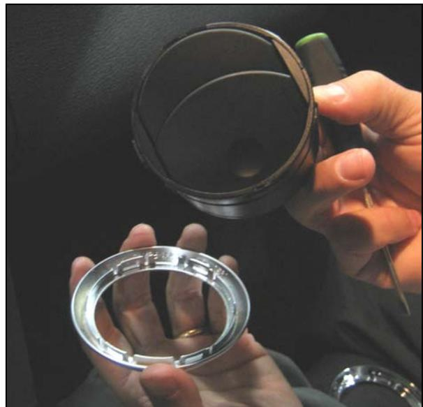
3. **THIS STEP IS FOR MUSTANG CUSTOMERS ONLY!** Using a set of side cutters, remove the F-150 bezel retainers (circled in RED in the picture below). You may need to file this area to ensure these surfaces are now flush with the outer bore.
