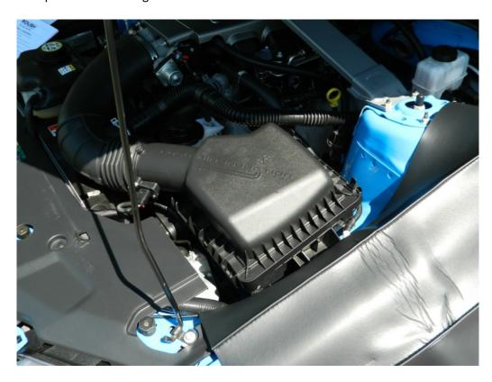
3. Using 5/16 socket and ratchet loose clamp that attaches inlet tube to air box lid and remove intake hose.
