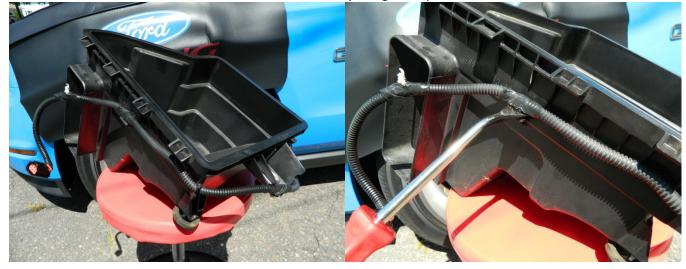
13. Remove body mount grommets from factory assembly.
