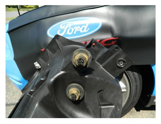
4. Install Roush air box assembly in to vehicle attach using oringal bolt tighten to 71 in-lb. using a 10mm socket.
