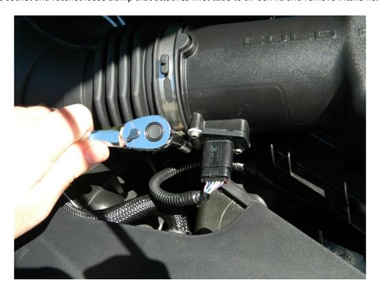
4. Disconnect mass air flow sensor wire harness at rear of air box.
