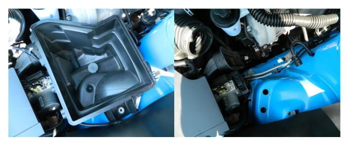
12. Remove mass air flow harness from lower air box assembly using a body trim removal.
