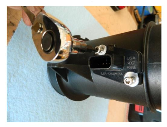
6. Install air filter to inlet tube using 5/16 socket and torque to 27 in-lb.
