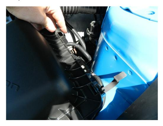
8. Remove mass air flow sensor from factory housing lid using T-20 Torx socket.
