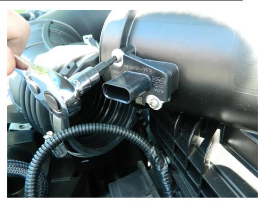
9. Using a body trim removal tool remove wiring harness from factory air box lid.
