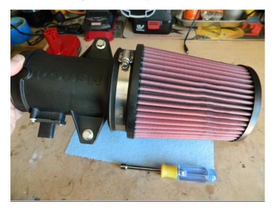
7. Attach factory intake hose to Roush mass air flow tube and tighen using 5/16 socket to 27 in-lb.
