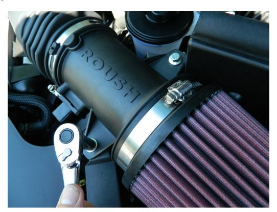
9. Reattach mass air flow sensor harness install connector until locks and then push in red safety tab. Run harness wire around to back and reattach to factory harness.
