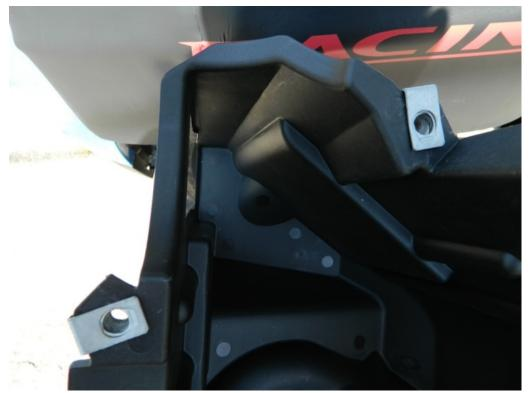
3. Re-attach original body mount grommets to Roush lower assembly.
