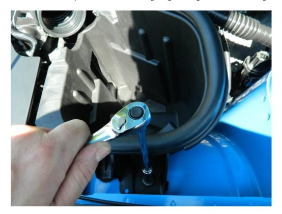
5. Install mass air flow sensor in Roush intlet tube with orginal hardware screws tighen to 16 in-lb.
