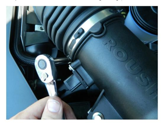
8. Secure Roush mass air flow tube to air box assembly using provied bolts, torque to 102 in-lbs using a 10mm socket.
