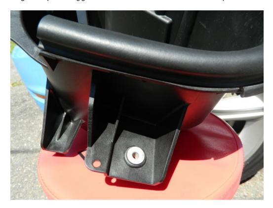
2. Install two J-clips to air box assembly.
