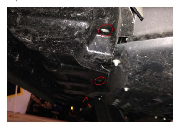
5: Along the front of the factory splitter, remove the 12-7mm bolts holding on the air deflector. 5 are shown below circled – the remaining 7 follow the same pattern along the front of the splitter.
