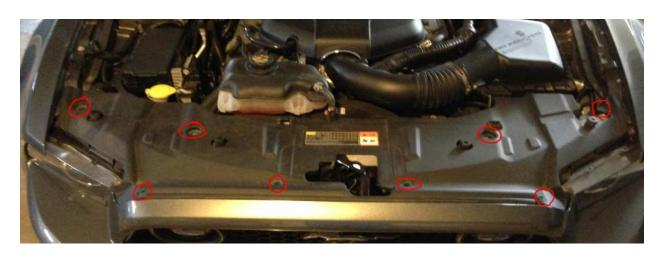
2: Remove the 4-8mm bolts and 4 plastic clips with a Philips screw driver. Each pair is circled below. Set aside for reinstallation.
