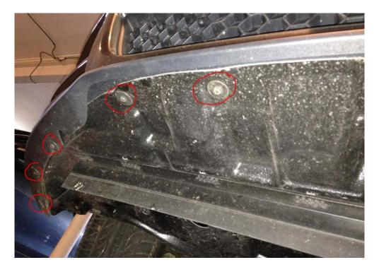
6: Slide the air deflector back and out of the way.
