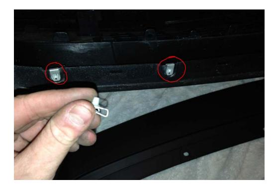
16: Temporarily install the new chin splitter to the bumper by attaching 4 bolts supplied – 2 in the middle U clips and 2 in the outside 2 clips installed in step 15.
