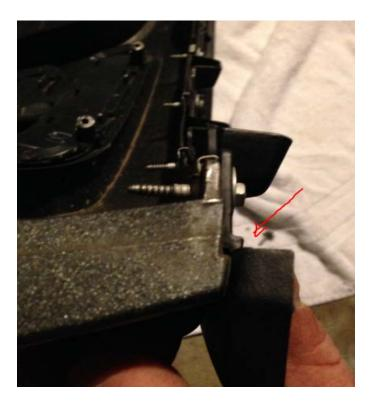
18: Using a 3/16" drill bit, drill through the outermost hole and attach the splitter to the bumper by using an attached U clip and bolt. This is the left circle in the picture below.
