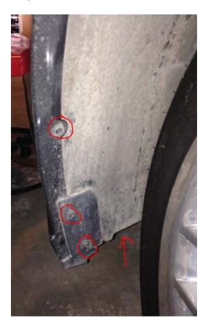
4: Remove the 3-7mm bolts attached the air deflector furthest back near the oil pan cover. 2 are circled below and the remaining is shown by the arrow below.
