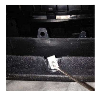
15: Attach 8 U clips supplied with the kit in the same spots as removed in step 14.
