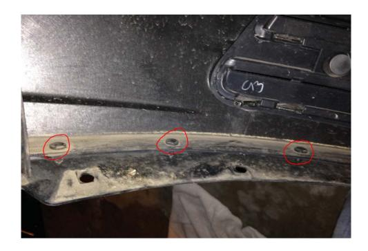
13: Remove the factory splitter by releasing the 6 clips in the middle inside of the bumper – 2 are shown below.
