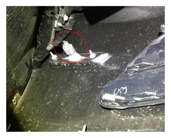
8: Unplug the ambient air thermometer by pulling downward.
