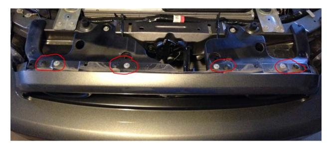
3: On each side, remove the 3-7mm bolts circled below attached the bumper on the front side of the wheel well. Remove 1-7mm bolt as shown by the arrow from the bottom of the wheel well closest to the outside.
