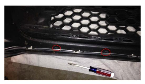
14: Remove the 8 U clips attached to the inside of the middle of the bumper.
