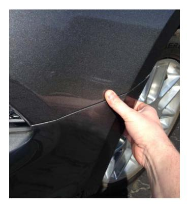
10: Holding the top of the bumper, pull out and down until the bumper is removed.
