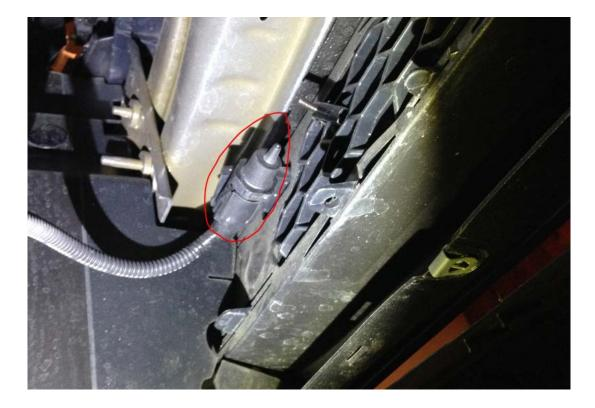
9: On each side, pull out on the top half of the bumper to remove the tabs holding it in place.
