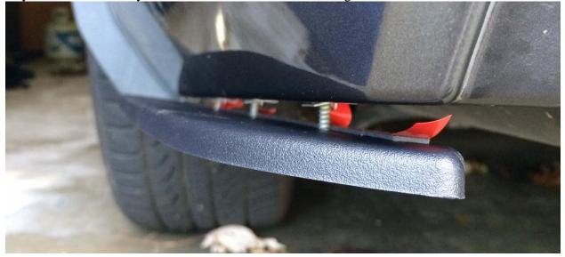
Step 13: If any clips are out of place or crooked, reattach or redrill holes as necessary.
