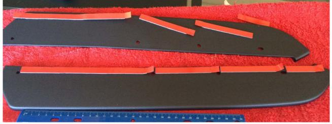
Step 10: Clean the bottom of the bumper (where the holes are drilled) with alcohol and remove any burrs from where the holes are drilled.
