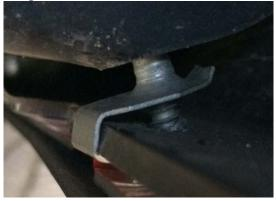
Step 14: Remove the red off the tape and tighten bolts all the way down. Step 15: Enjoy!
