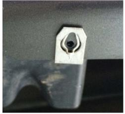
Step 12: Take the splitter labeled LH and loosely attach the screws to the driver's side J clips. Take the splitter labeled RH and loosely attach to the passenger's side. Do not attach all the way, as this will allow you to check fitment before finalizing installation.
