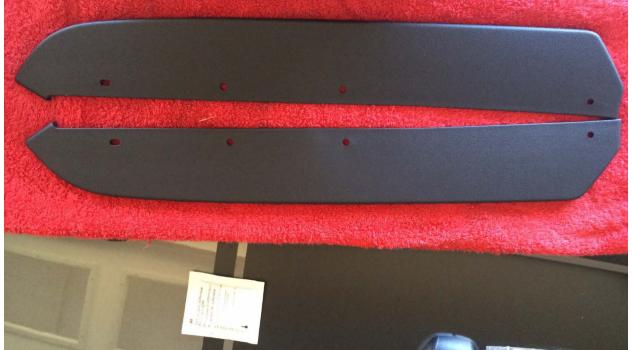
Step 7: Clean the top of the splitters with alcohol. This will allow the tape to attach.
