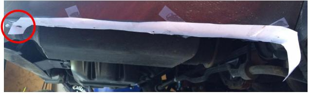
Step 4: Take the driver's side splitter (labeled LH on the bottom) and check to see if all holes are aligned. Also check for fitment of the splitter along the bumper. If anything is out of align, reposition the template.
