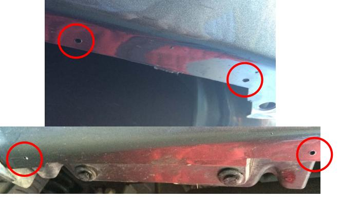
Step 5: Using the 1/8" drill bit, drill through the paper template where marked in the 4 spots.
