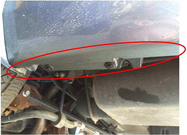
Step 3: Starting on the driver's side, tape the template along the bottom side of the bumper. Line up the hole punched in step one first and follow along the edge of the bumper back towards the wheel.
