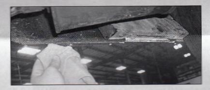
2. Install the four (4) J-clip fasteners (W704823-S439) into the 1/4" drilled holes.
