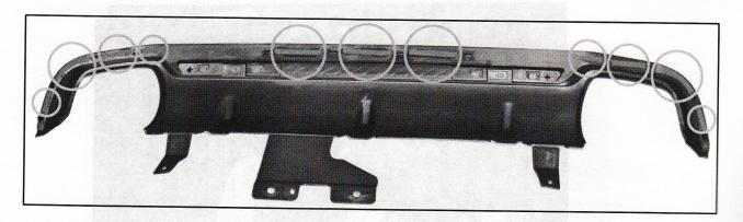
27. Peel the backing off the 2-sided tape.
