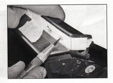
13. Remove the template, use a 1/8" drill bit to drill the pilot holes and finish with a 1/4" drill bit.
