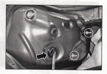
5. Remove the six (6) screws and depress the two (2) center clips on the LH and RH side splash shields to release.
