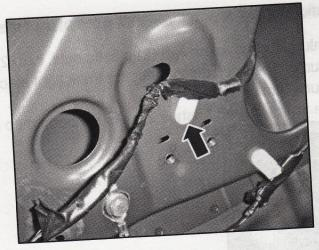
3. Disconnect the LH and RH tail lamp electrical connectors.
