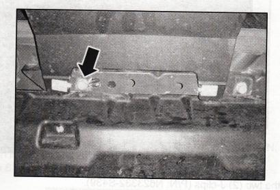
3. With the bumper cover installed, mark the center of the two (2) holes for the center bumper cover mount.
