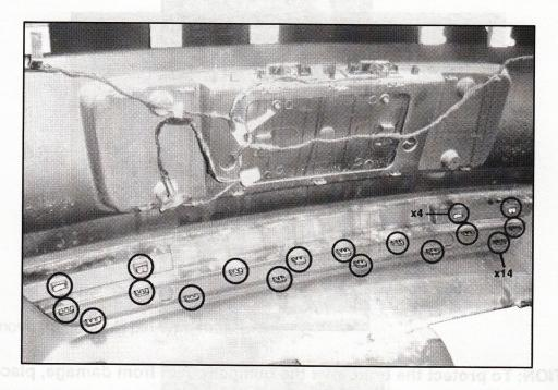
11. Cut out the exhaust area templates provided in the kit (P/N: 1313-17F958TMPL), tape the template to the bumper cover and mark the area as shown.
