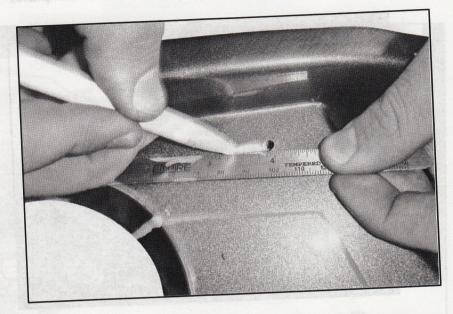
15. Using a 1/4" de-burring tool, open the slots marked on the bumper.
