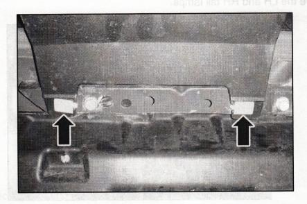
7. Remove the four (4) pin-type retainers.
