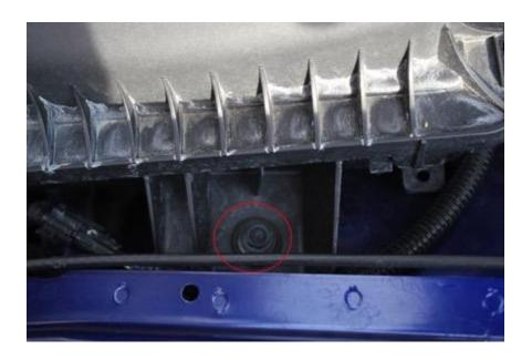
Pull air box up to release from grommet from bottom of air box. Remove air Intake system from car.
