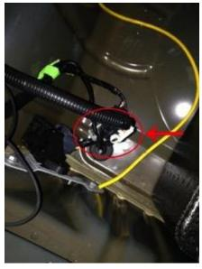
With wiring up under the sill of the trunk plug the Roush Instrument box in, and screw it in with the 4 self tapping screw supplied above the rear fender, located the hole in the sheet metal and place it over the hole, use a ¼ socket to secure the box.
