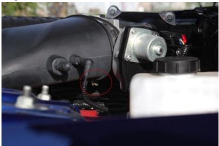
Loosen 8mm bolt clamp on bottom air box side. (Red Highlight) And remove the Mass Air Flow Sensor with a T20 TORX screwdriver. (Green Highlight) set aside for new intake. Image below:
