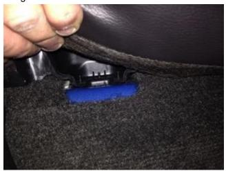
Remove drivers side sill panel, by pulling up on the outer edge, but be sure to disconnect the illumination wiring.
