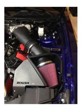
Install new air box and clamp it on throttle body. With the 8mm Hose Clamp. Image below:
