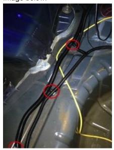
Locate the Fuel Pump Module, at rear of spear tire hole on drivers side, unplug the harness and plug the splitter wire in and plug harness into splitter.
