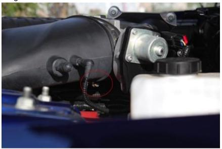
Under the Roush letter on air box, there a slot for a bolt to go through on radiator, and there is a nut supplied with the bit, also a 8mm.
