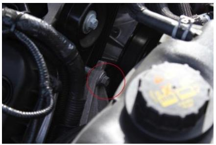
(You may need to take other 2 bolts loose on Idler bracket to allow movement) Slide the new (2085 6 Rib) Belt On.
