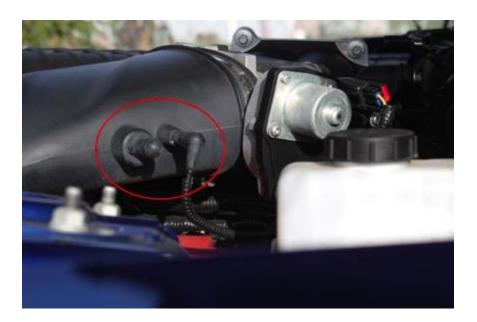
Remove the 10mm Bolt on Drivers side between fender and air box. Image below:
