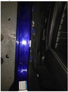
Remove the Drivers side kicker panel by using a trim too on the small clip holding it in place Pull carpet up so it exposes factory wiring.
