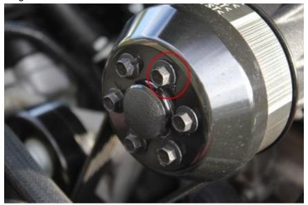
Use a Pulley Puller tool, to remove stock pulley.
