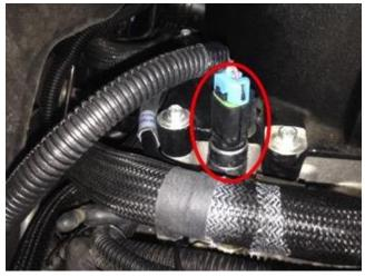
Thread the switch into intake hole we removed boost line from earlier.
