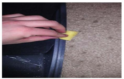
3. Next you will need to apply the 3M tape to the louver. The 3M tape is precut to fit the louver so it should be pretty straight forward to see where each should be attached.
