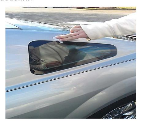
6. Now you're ready to mount the louver to the car. Peel back the red adhesive tape off the louver and place it in its desired location.
