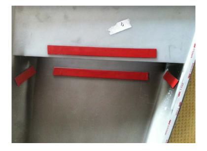
15. Remove the backing from the tape and press the grille firmly into place.
