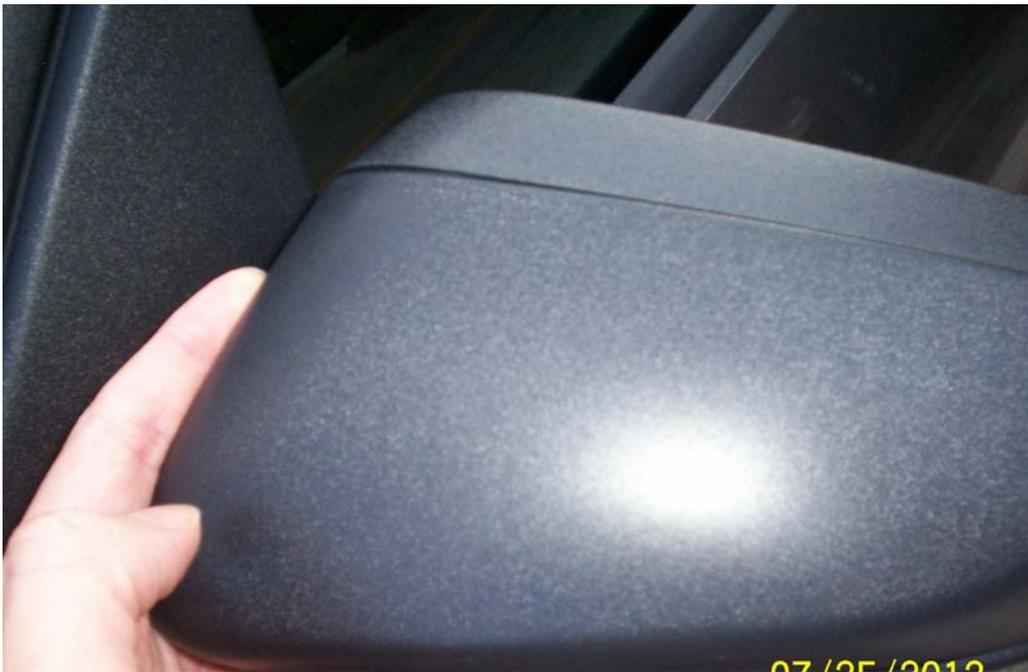
3. Using both hands apply firm pressure pulling into your body and up at the same time. *These mirror covers are held in by one large push in snap lock type connector. By pulling towards you and up at the same time you will pop this connector off.*
